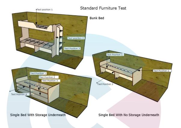
NB Test point 1 on the bunk bed is to simulate someone attempting to kick the arrester panel off and should be carried out as if the force is coming from someone on the bed.
